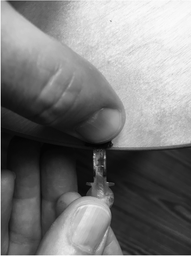
Photo 1. Press downwards with the right thumb, the plate which carries the pad is pressed flat on the edge of the table.
